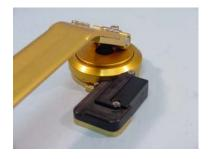
**SJ92** LTI Locking Shoulder Joint, Endoskeletal, Electric Lock Actuator This joint has an electric lock actuator For electric lock actuation, a cable, switch, battery and charger are required The joint is supplied with the exoskeletal plate attached.
